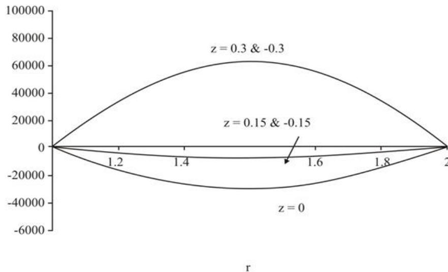
**Figure 5: Tangential stress distribution along radial direction**
