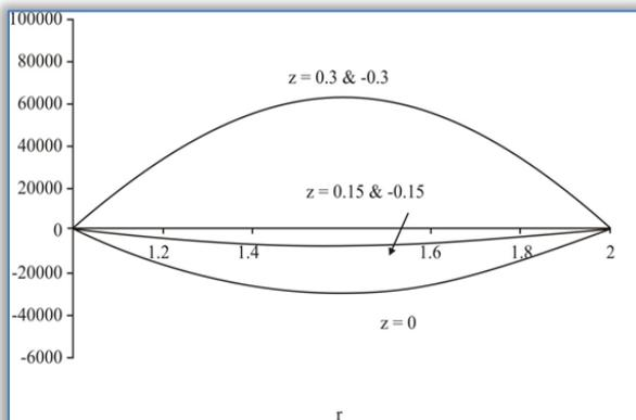
Figure 5: Tangential stress distribution along radial direction
