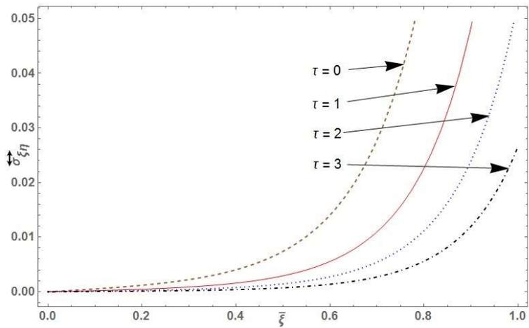
Fig. 5(c). Shear stress  $\bar{\sigma}_{\xi\eta}$  along  $\bar{\xi}$  for different values of  $\tau$
