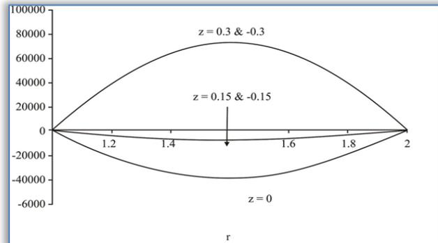
Figure 4: Radial stress distribution along axial direction
