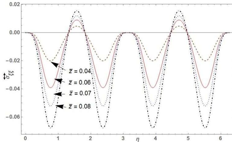
Fig. 3(b). Dimensionless radial stress along  $\eta$  for various values of  $\bar{z}$
