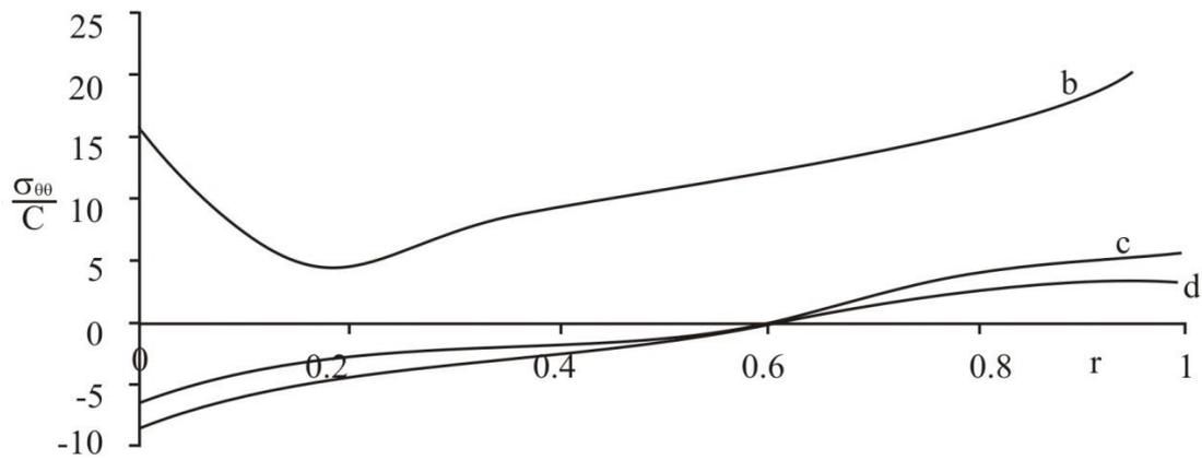
Figure 6. Tangential stress distribution
