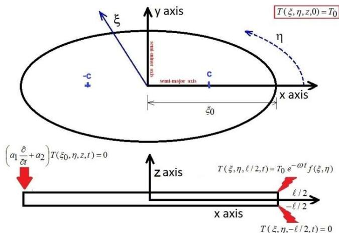
Fig. 1. Physical configuration of the elliptical plate
