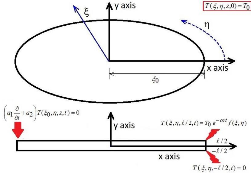
Figure 1. Physical configuration of elliptical plate
