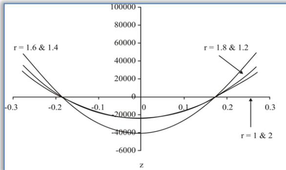
Figure 3: Radial stress distribution along radial direction
